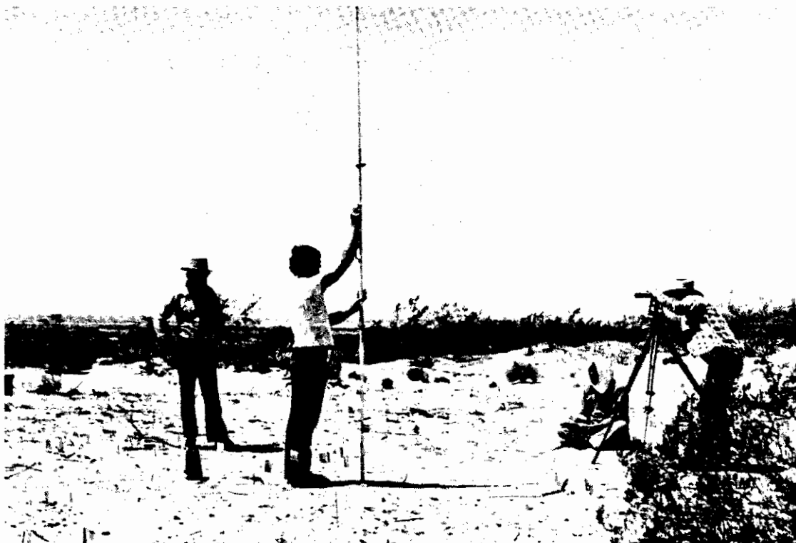
FIGURE 3 The four person artifact piece-plotting team at work at FS1, in the proposed Golf Resort Joint Venture Subdivision, El Paso, Texas. It was possible to piece-plot 60 or more artifacts per hour with one person on the transit, one person recording angle and distance information, one person holding the stadia rod, and one person cataloging the artifacts. Over 90% of the 1129 artifacts piece-plotted in the FS1 assemblage were taped in; the distance to the remaining surface artifacts were determined by reading stadia. Use of a stadia rod permitted elevation determination at each artifact loci, facilitating site map preparation, as well as assisting aspects of the subsequent analysis focusing on possible post-depositional disturbance or spreading patterns.
